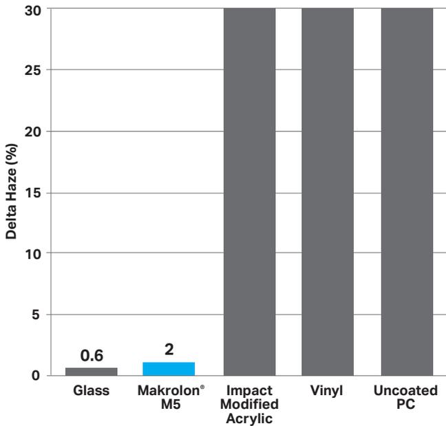
\*Taber Abrasion per ASTM D 1044, 100 cycles, CS-10F wheels at 500 g load
